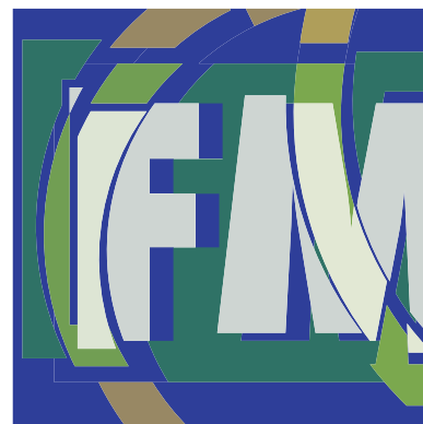
Flattened art simulates transparency by cutting up objects (objects slightly shifted for illustrative purposes)
