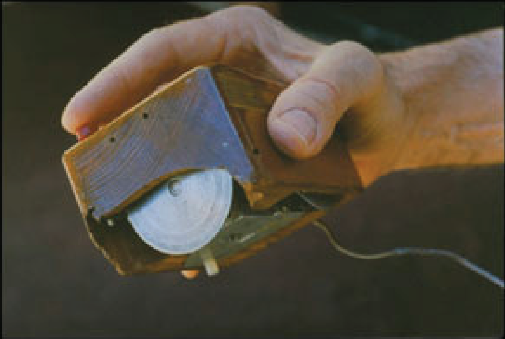
The first mouse, a small wooden box on steel wheels, was invented by scientist Douglas C. Engelbart in the 1960s at the federal government's Augmentation Research Center
